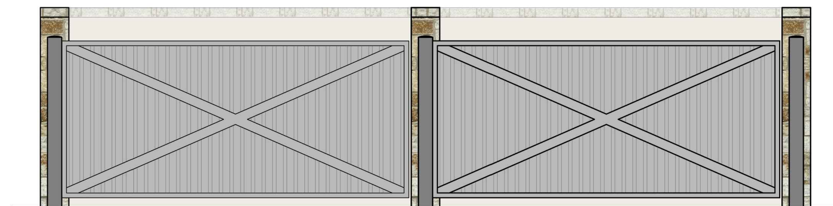
3 DUMPSTER ENCLOSURE FRONT ELEVATION 1/2" = 1'-0"
