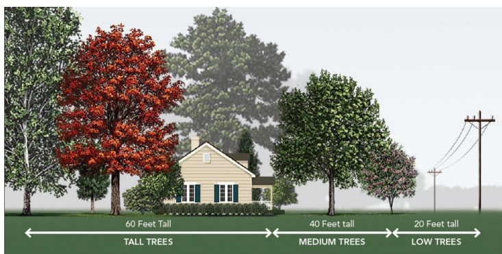
Figure 2. Buffer Distances from Utilities
